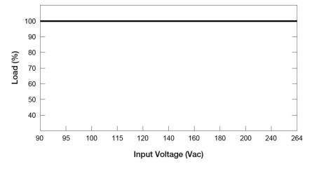
No output power de-rating for the input voltage from 90Vac to 264Vac
