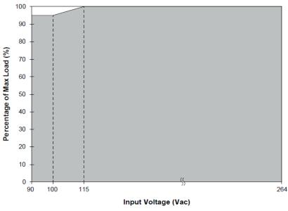
Fig. 4.2 De-rating for Horizontal Base Mounting Open Frame (PJU-13V)
