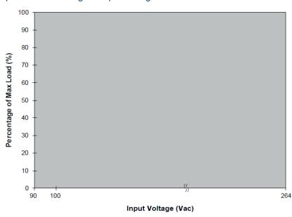
No output power de-rating for the input voltage range, refer to Fig. 4.1.
